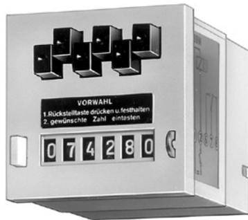
The electromechanical preset counters MVs 16 (with manual and electrical reset) boast a robust construction. They are ideal for use in harsh industrial environments. The subtracting counters are set to a value via the keys on the front, the signal occurs when the count value reaches 0.
