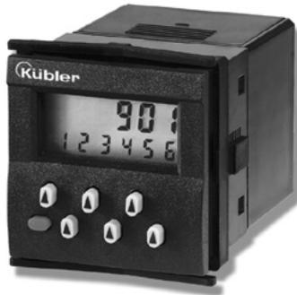
Type 901 is a simple battery-powered preset pulse counter/timer with 12 ... 250 V AC/DC count and reset inputs or with NPN input. The 6-digit, 2-line LCD display shows the current count value, the preset value, the relay state and the active time measurement.
