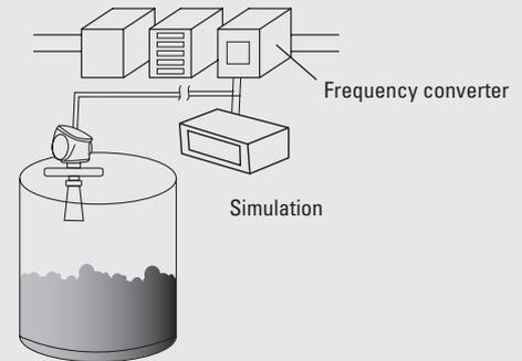
Alignment for temperature-based processes without having to heat up the plant: the setpoint adjuster can simulate various processes for test purposes.
