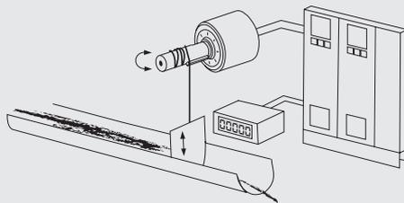
Calibration of filling levels and flow rates: the setpoint adjuster simulates the output signals of a level or flow sensor for configuring a control.
