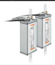
Ants LEB02 is an extremely robust, compact and contactless measuring system. It uses a contactless measuring principle to measure without any slipping absolute elevator car positions with a resolution of 1 mm and a travel speed of 8 m/s. Additional components such as magnetic switches become superfluous. Especially the easy assembly reduces installation time, thus contributing to overall costs reduction.
