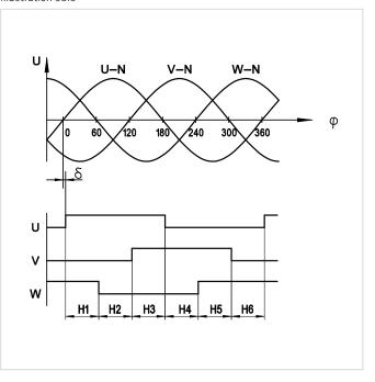
$$\begin{split} T &= 360^{\circ}/2000 \\ a, \ b, \ c, \ d &= 0,25\ T \pm 0,15\ T \\ Tz &= T \pm 0,5\ T \\ HN &= 360^{\circ}\ /\ 5\ /\ 6 = 12^{\circ} \\ \delta &\leq \pm 3^{\circ}\ el. \end{split}$$
