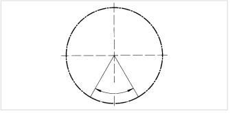
At oscillating angles < 5° fretting corrosion may occur due to insufficient lubrication. In this case please contact our sales engineer for countermeasures
