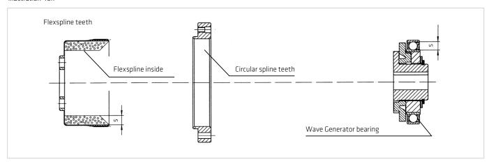
The required amount of grease is dependent on the size and the operating position of the gear. The operating positions "Wave Generator above" or "Wave Generator below" refer to the relative position of the Wave Generator to Flexspline flange, see illustration 48.2.
